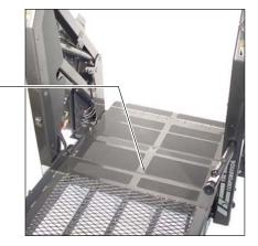
the UP switch is pressed and the platform raises from ground level, the inboard locator automatically unfolds (rotates) to the horizontal (bridging) position when it reaches vehicle floor level. The bridge plate must overlap the lift base plate a minimum 1/2".
